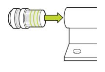
Use the insert required with lock nut
