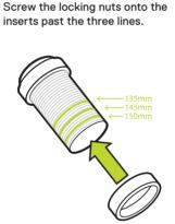
2 Screw the insert into the base up until the desired width line is flush with the base. 135 (outer line), 145 (middle line) and 150 (inner line).
